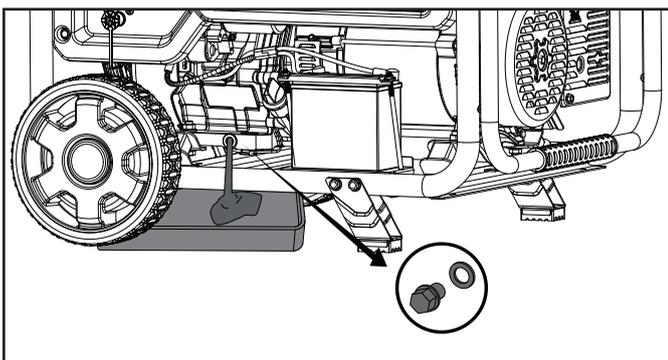
3. Replace the oil drain bolt.
