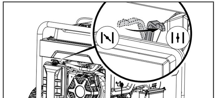
9. Press and hold the ignition switch in the “START” position for up to 5 seconds or until started.
