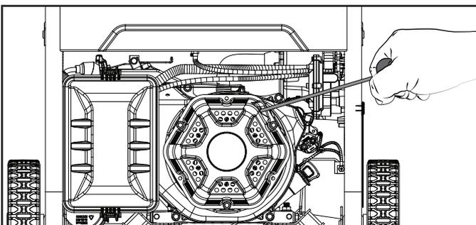
10. When the engine starts, move choke to the "RUN" position if in the "CHOKE" position.
