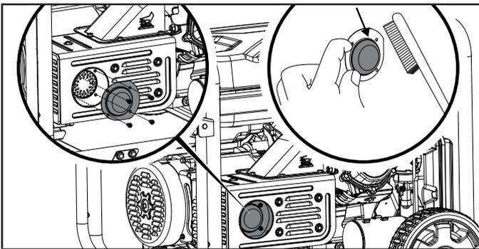
5. Replace the spark arrestor if it is damaged.
