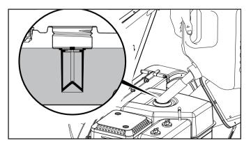
3. Screw on the fuel cap and wipe away any spilled fuel.
