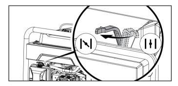
5. Fully open the valve on the LPG cylinder.
