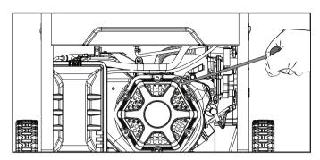
2. Move the choke lever to the "RUN" position.
