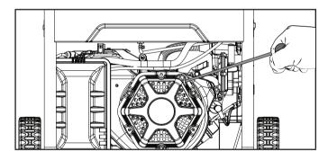
4. If engine fails to start in 1-pull with choke in the "RUN", then move choke lever to the "CHOKE" position and repeat the PULL-TO-PRIME step.
