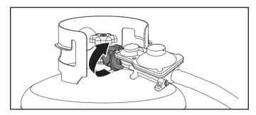
6. Check all connections for leaks by wetting the fittings with a solution of soap and water. Bubbles which appear or bubbles which grow indicate that a leak exists. If a leak exists at a fitting then turn off the valve on the cylinder and tighten the fitting. Turn the valve back on and recheck the fitting with the soap and water solution. If the leak continues or if the leak is not at a fitting then do not use the generator and contact customer service.
