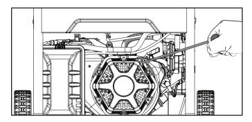
2. Do not over-choke. As soon as engine starts, move the choke lever to the "RUN" position over a 2-5 second duration.
