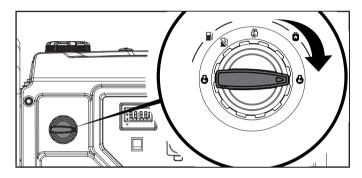
4. Move the choke lever to the "CHOKE" position.
