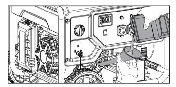
4. Check engine oil level at every use and add as needed.
