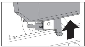
3. Pull out the spring loaded quick-lock pin and rotate it around to the 9 o'clock position around the lip on the beam to secure it in the vertical position.
