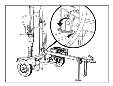
4. To change from vertical to horizontal orientation, reverse the steps. The beam will automatically lock into the auto-lock on the tow bar when lowered into position.
