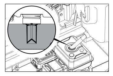
The approximate fuel level is shown on the fuel gauge on top of the fuel tank.
