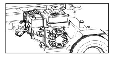
As engine warms up, move the choke lever to the "RUN" position.
