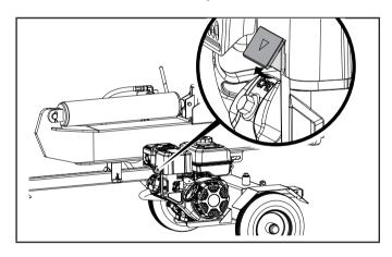
2. Remove both air filter cover and air filter element.
