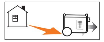
If misused and operated in an unapproved and unsafe location that results in the accumulation of poisonous CO gas inside an enclosed or partially enclosed space, for example a house, garage or a garage with the door partially open, CO Shield<sup>®</sup> will automatically shut off the generator and then will illuminate a blinking red LED light. **Read the action label for next steps.**
