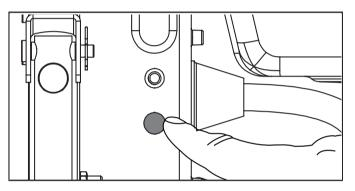
4. Push and release the STOP 🖏 button on the remote key fob. The red light blinks once to erase the remote program.
