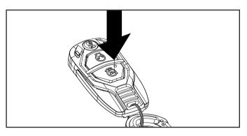
5. Push and release the START **b** button on the remote key fob. The red light blinks once to program the remote.
