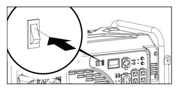
Press and hold the ignition switch to the "START" position. Release as the engine begins to start. If the engine fails to start within five seconds, release the switch and wait at least ten seconds before attempting to start the engine again.
