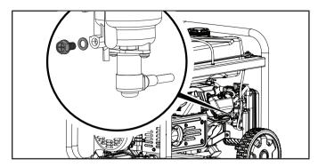
5d. When gasoline stops flowing from the carburetor, replace and tighten the carburetor drain bolt and be sure to properly dispose of the drained gasoline according to local regulations or guidelines.
