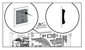
Press and release the "START" button on the remote key fob. D0 NOT hold the button down, only press the button once. The engine will attempt to start six times.
