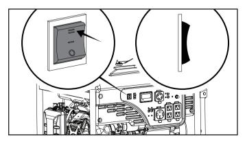
2. Turn the battery switch to the "ON" position.
