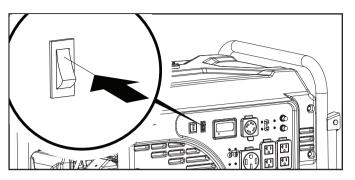
2. Push the ignition switch to the "ON" position.
