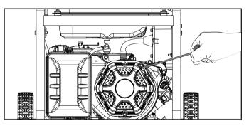
5. Do not over-choke. As soon as engine starts, move the choke lever to the "RUN" position over a 2-5 second duration.
