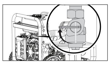
**Important:** Always ensure that the fuel valve, the ignition switch, and the battery switch are in the "OFF" position when the generator will not be used for an extended period of time.
