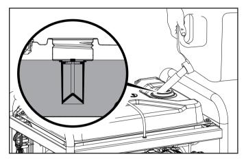
3. The approximate fuel level is shown on the fuel gauge on top of the fuel tank.
