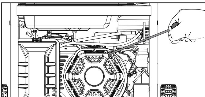
6. Do not over-choke. As soon as engine starts, move the choke lever to the “RUN” position over a 2-5 second duration.
