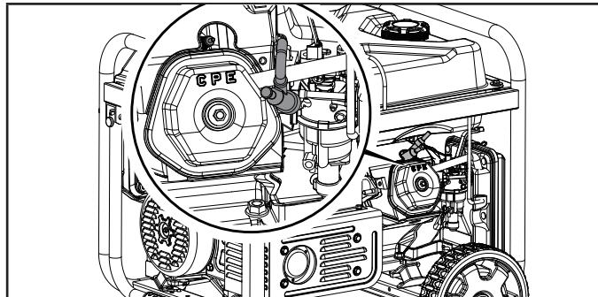
3. Inspect the electrode on the plug. It must be clean and not worn to produce the spark required for ignition.
