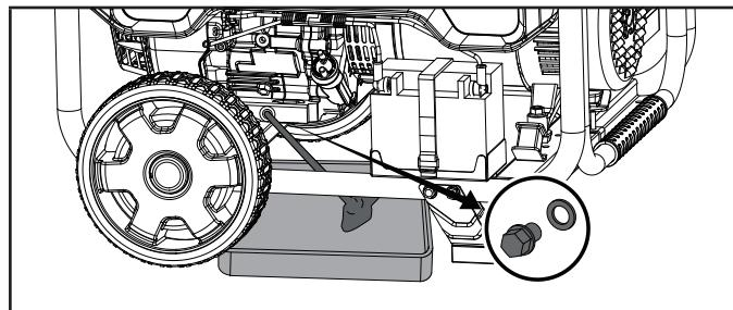
3. Replace the oil drain bolt.
